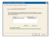
This screen shows the currently connected devices (excluding the local device) and their individual bit rates, this is useful for diagnosing slow transfer speeds. The connection speeds are updated when this screen is selected and then again when the 'Scan Powerline Network' button is pressed.
